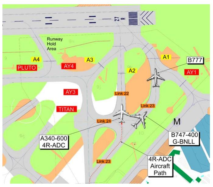
**Figure 1**Point of collision at holding points for Runway 27R
