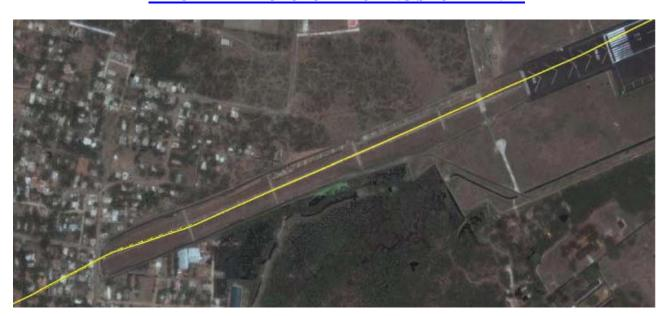
TRAJECTORY OF LEFT MAIN LANDING GEAR ON THE RUNWAY 07
