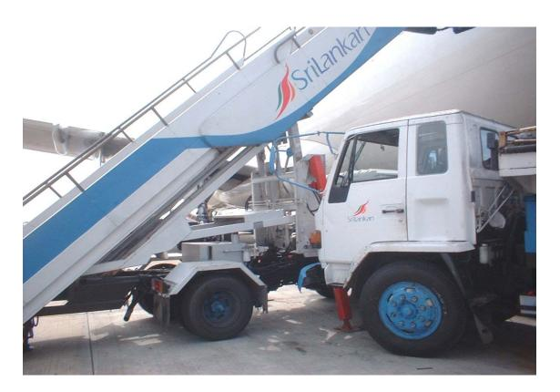
The Maintenance Step vehicle stopped after colliding with the stepladder
