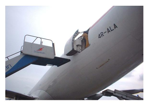
The gap created between the aircraft and the displaced stepladder
