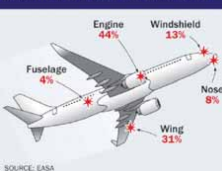
LOCATION OF BIRD STRIKE DAMAGE
