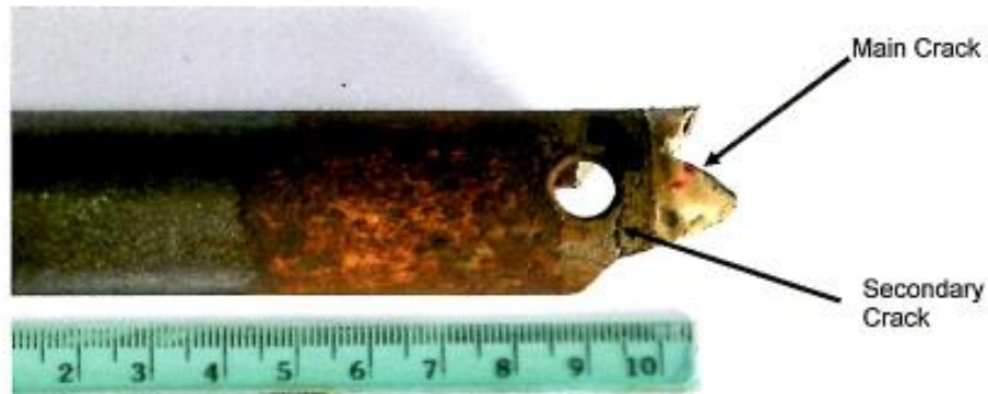
Figure 8: Other side of the Fractured Strut with the Cracks
