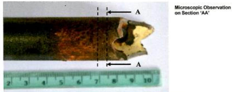
Figure 10: Sample Selection for the Metallographic Investigations
