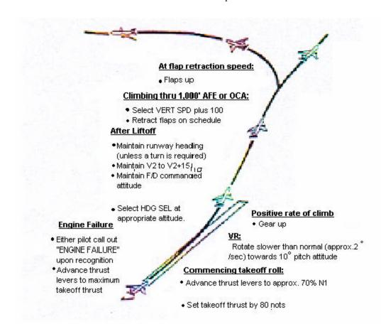
Note: Above procedure and settings relevant to operators aircraft AOM
