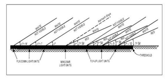
Figure 5-18. Light beams and elevation settings of T-VASIS and AT-VASIS
