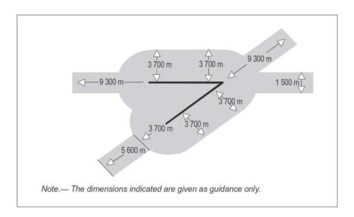
Figure 5-12. Multiple runway laser-beam free flight zone
