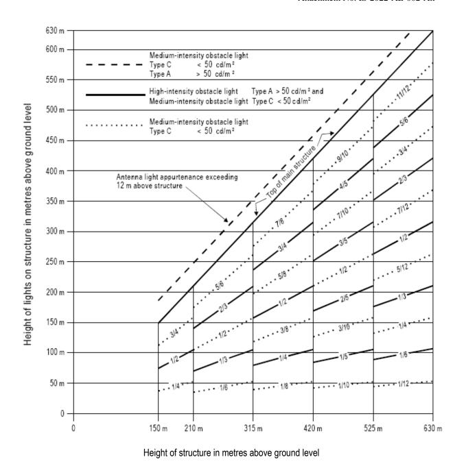
Figure A5-7. High-/medium-intensity dual obstacle lighting system, Type A/Type
