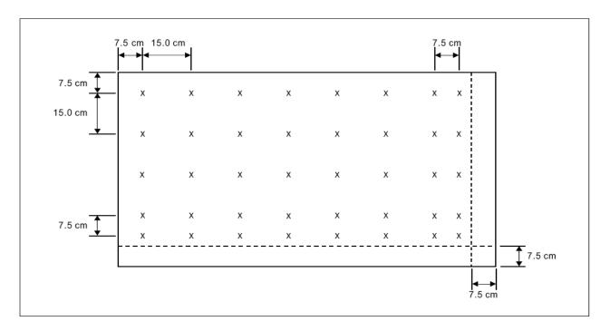
Figure A4-1. Grid points for calculating average luminance of a sign
