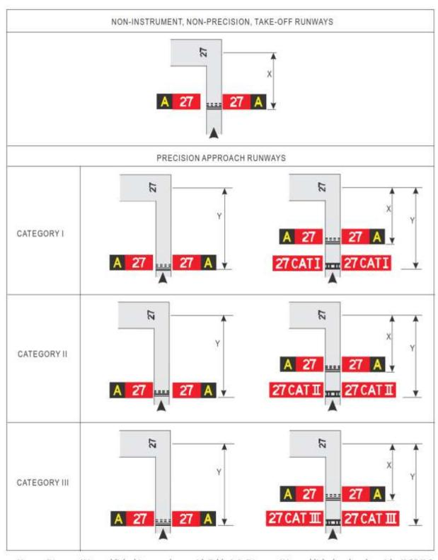
Note.— Distance X is established in accordance with Table 3-2. Distance Y is established at the edge of the ILS/MLS critical/sensitive area.
