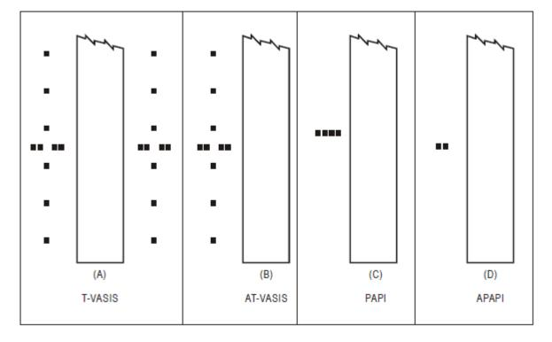
Figure 5-16. Visual approach slope indicator systems
