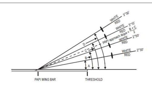
The height of the pilot's eye above the aircraft's ILS glide path/MLS antenna varies with the type of aeroplane and approach attitude. Harmonization of the PAPI signal and ILS glide path and/or MLS minimum glide path to a point closer to the threshold may be achieved by increasing the on-course sector from 20' to 30'. The setting angles for a 3° glide slope would then be 2°25', 2°45', 3°15' and 3°35'.
