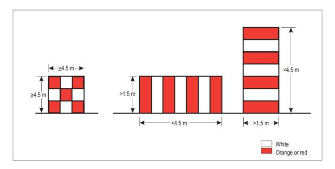
Figure 6-1. Basic marking patterns
