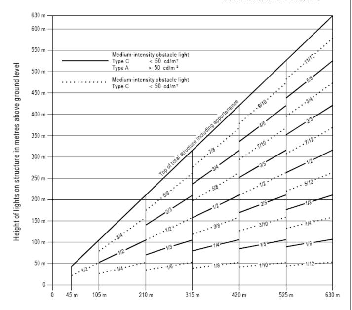
Note.— High-intensity obstacle lighting is recommended on structures with a height of more than 150 m above ground level. If medium-intensity lighting is used, marking will also be required.
