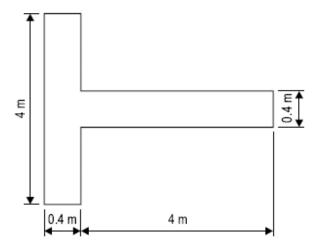
Figure 5-1. Landing direction indicator
