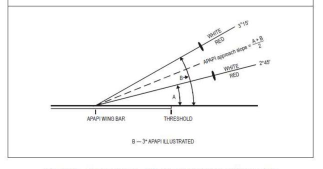
Figure 5-20. Light beams and angle of elevation setting of PAPI and APAPI
