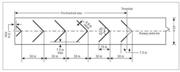
Figure 7-2. Pre-threshold marking
