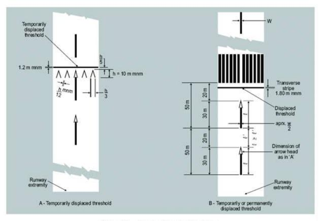
Figure 5-4. Displaced threshold markings
