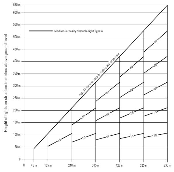
Note.— High-intensity obstacle lighting is recommended on structures with a height of more than 150 m above ground level. If medium-intensity lighting is used, marking will also be required
