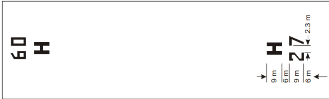
Figure 5-3. FATO designation marking and heliport identification marking for a runway-type FATO
