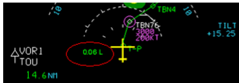
Figure 18.2: Lateral deviation displayed on a navigation (map) display
