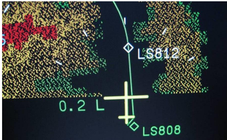
Fig 7.2: Example of cross-track deviation display in 1/10 th NM
