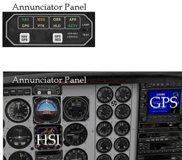
Figure 17.5: Typical Stand-alone GNSS installation
