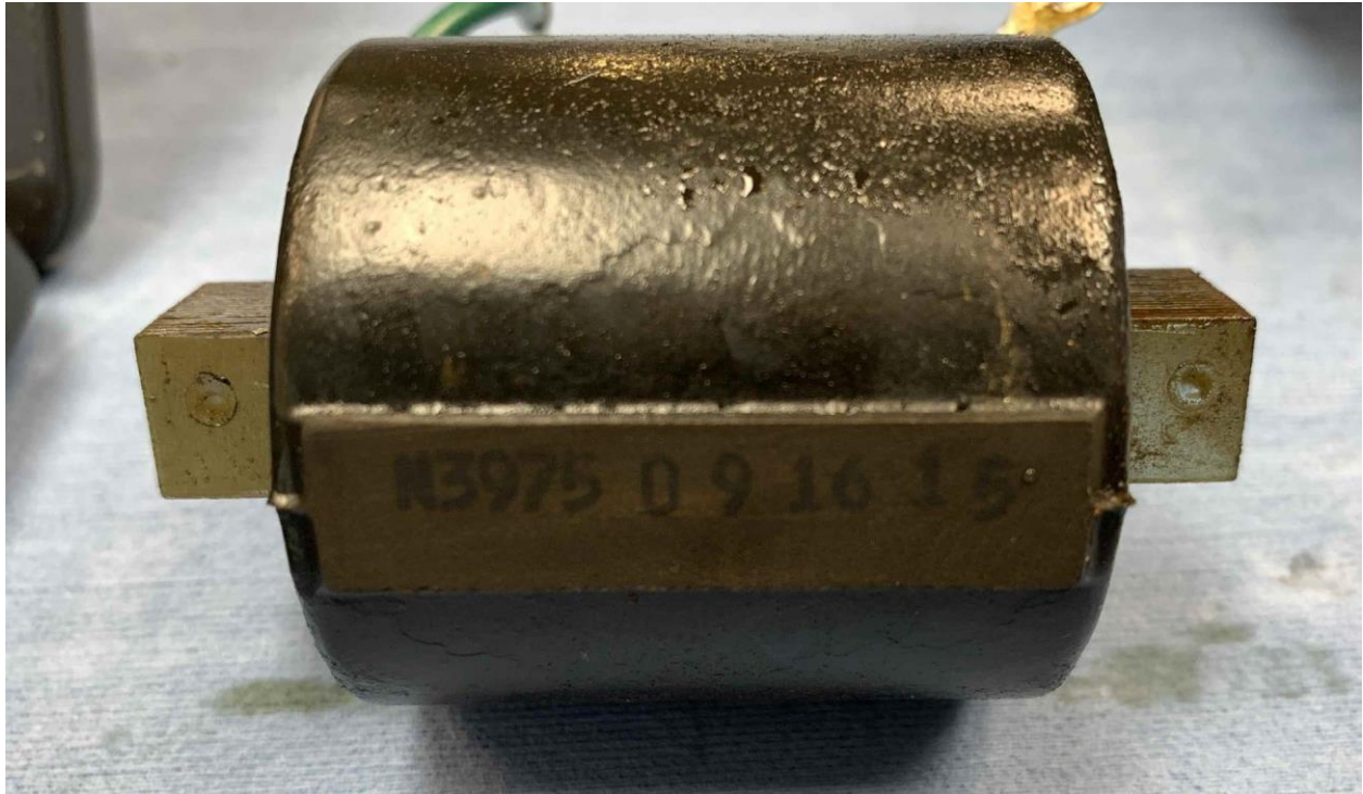
Figure 5 – Coil with data code
