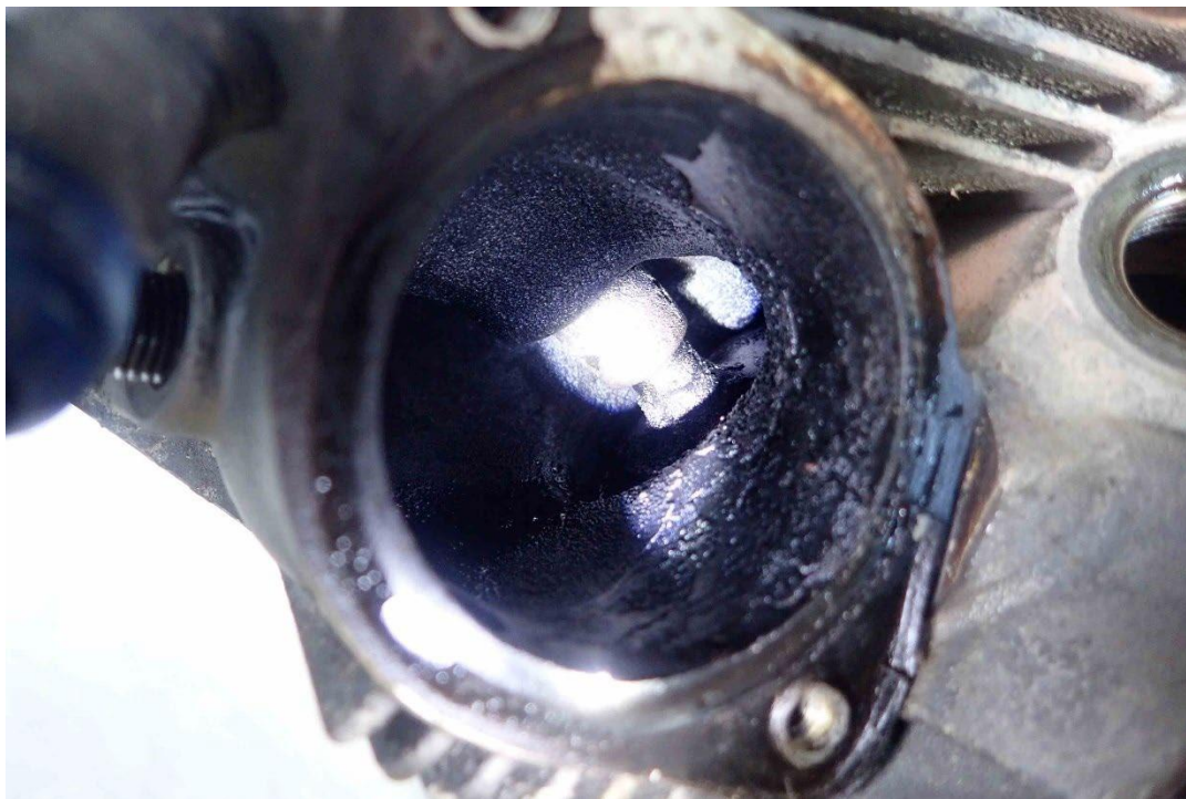
Figure 7 – Intake cylinder valve guide stem and back of valve face
