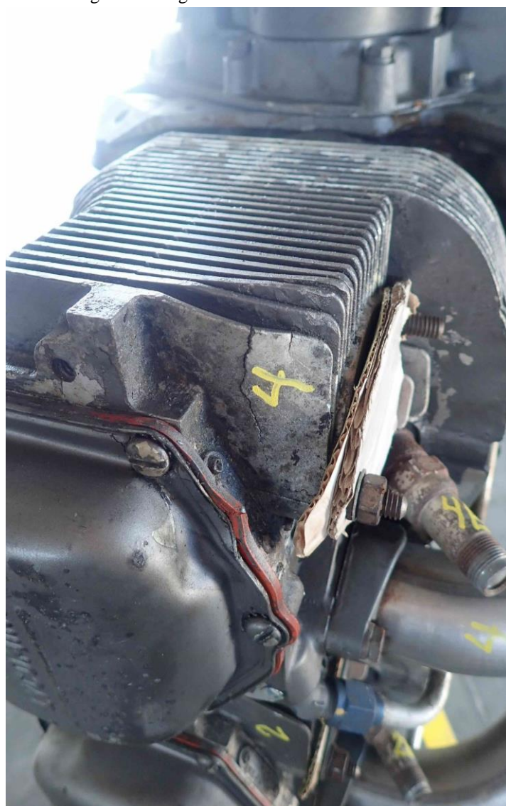
Figure 2 – Number 4 cylinder fin damage
