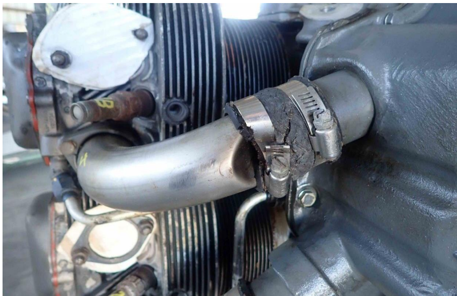
Figure 3 – Number 4 cylinder inlet manifold damage
