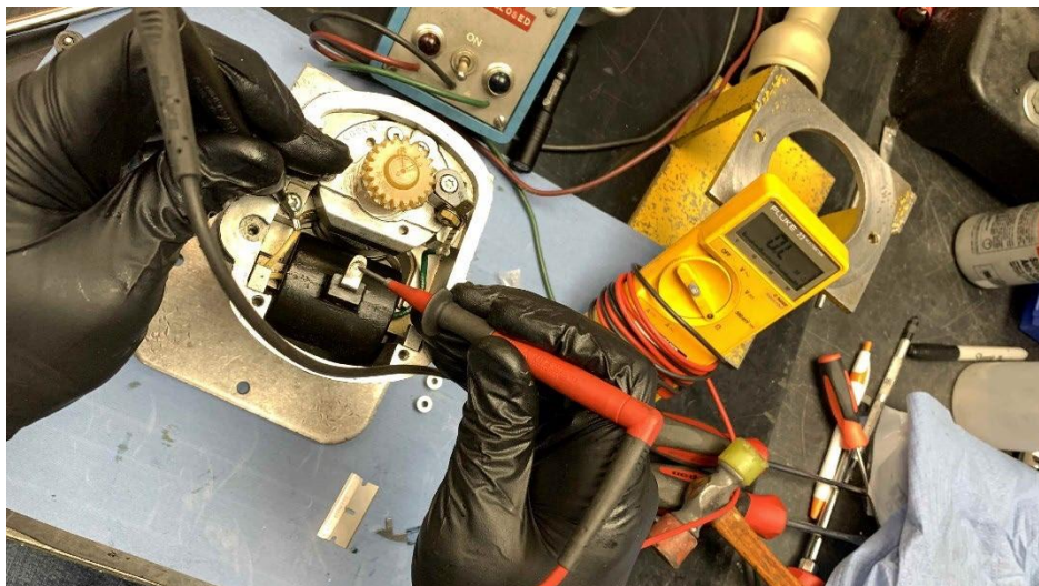
Figure 3 – Coil secondary winding resistance
