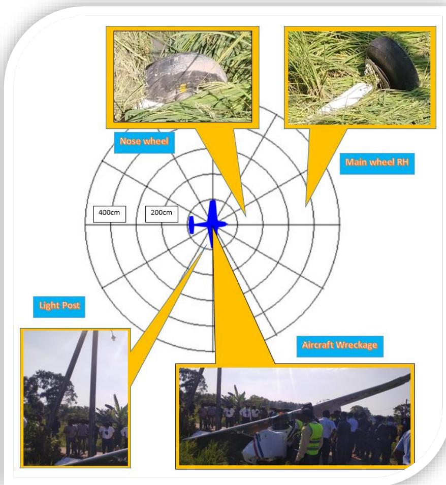
Figure 09: Wreckage distribution chart
