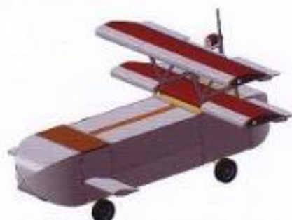
"The figures show the 1:5 scale radio control model which is currently being developed to be used as a test bed for trying out various aerodynamic design concepts."
